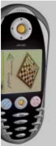
Atelab's Chameleon operates in two positions; vertical as a mobile phone and horizontal as a game console
