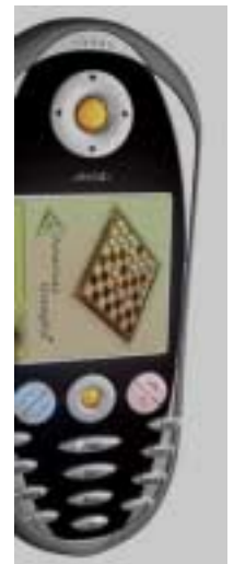
Atelab's Chameleon operates in two positions; vertical as a mobile phone and horizontal as a game console
