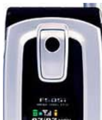
F505i with fingerprint sensor (DoCoMo)
