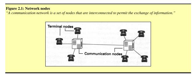
So a network consists of nodes and interconnections. Nodes can be of two types, terminal nodes and communication nodes. Terminal nodes generate or use information on the network.
