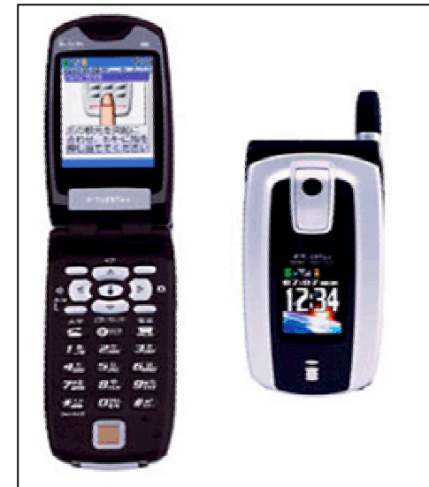
DoCoMo F505i With fingerprint sensor
