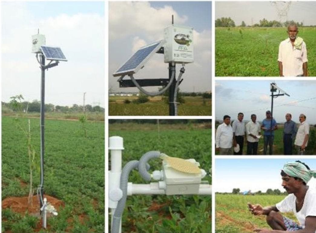
Figure 1 – Harita-Priya – Collage: Open field deployable WSN node, communication unit and sensor unit
