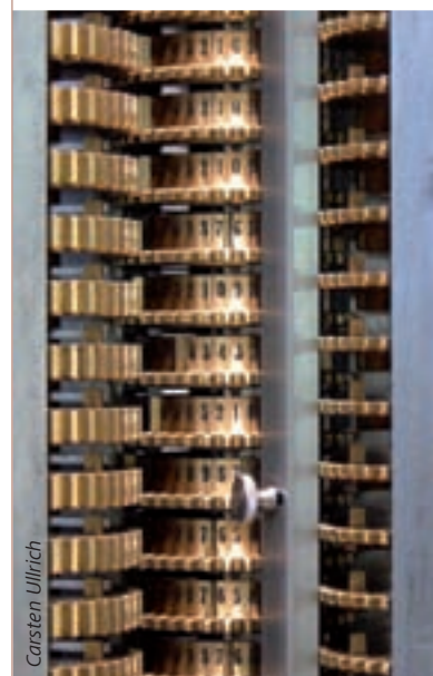
Close-up view of the Difference Engine, showing the figure wheels arranged in columns
