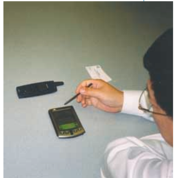
Mobile phone connected to a Palm Pilot PDA via infrared being used to dial-up Internet (Singapore)
