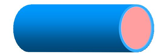
Paper insulated buried cable: 400 pairs conductor diameter: 0.40 mm shield resistance:  $1.1 \Omega / km$
