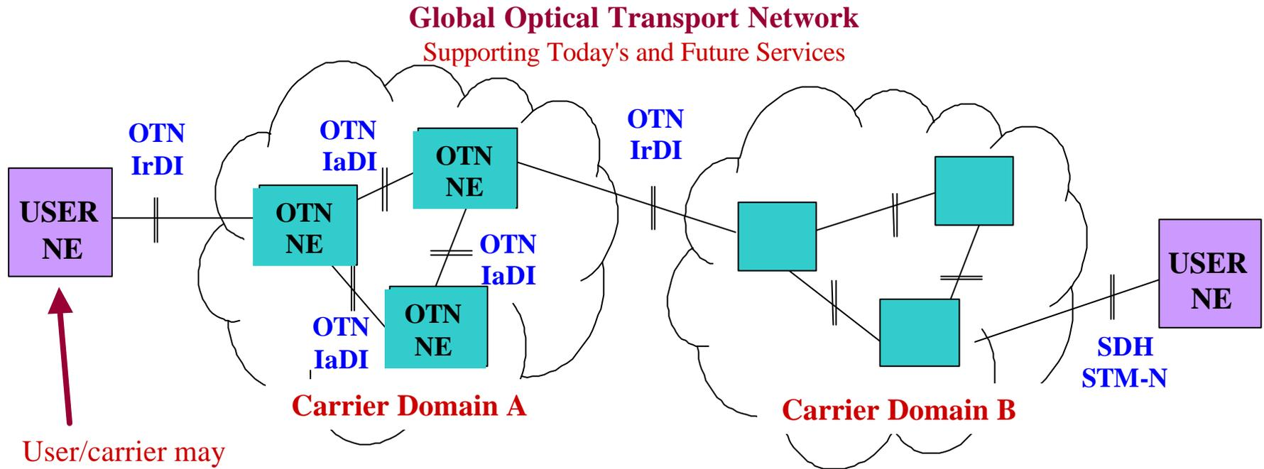
User/carrier may originate/terminate the OTN framing for any digital payload (IP, ATM, SDH,,)
