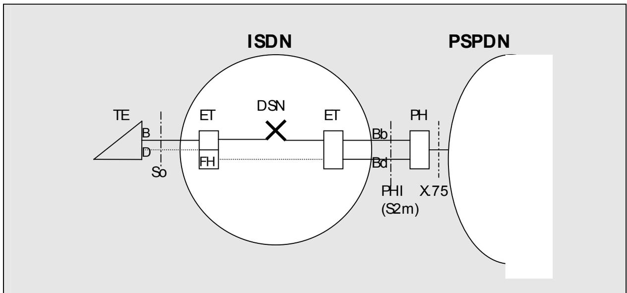
In the ETSI scenario the PH-function is located outside the ISDN, often close to the PSPDN, but still logically belonging to the ISDN. The PH is accessed via a standard Packet Handler Interface, PHI, which is physically an ISDN Primary Rate Interface.
