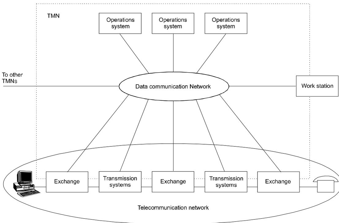
TMN is intended to manage all kinds of telecommunication equipment (e.g. transmission and switching equipment), telecommunication support equipment (power supply, air conditioning and security equipment) and itself. TMN as a tool supports network operators and intends to offer easy to understand human/machine interface routines. The broad concept of TMN can be described using different architecture aspects (see Table 5.2).
