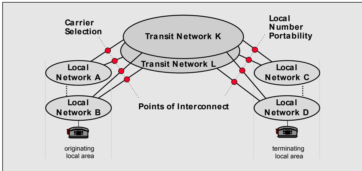
As indicated in the Figure 2.7.3, in case of a long distance call, carrier selection determines the call routing towards and interworking at the point of interconnection in the originating local area. In the terminating local call area, number portability requires new routing methods to select the point of interconnection to and appropriately inter-work with destination local networks.
