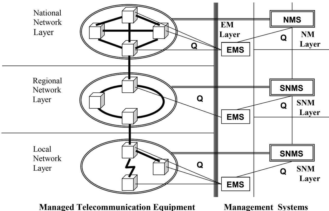
Depending on the hierarchy of networks, e.g. local, regional and national networks, a hierarchy of corresponding Network Manager Systems can be defined leading to the number of Subnetwork Manager Systems (SNMS), which are hierarchically connected to NMS. An example deployment of MS for transport network is shown in Figure 5.7.
