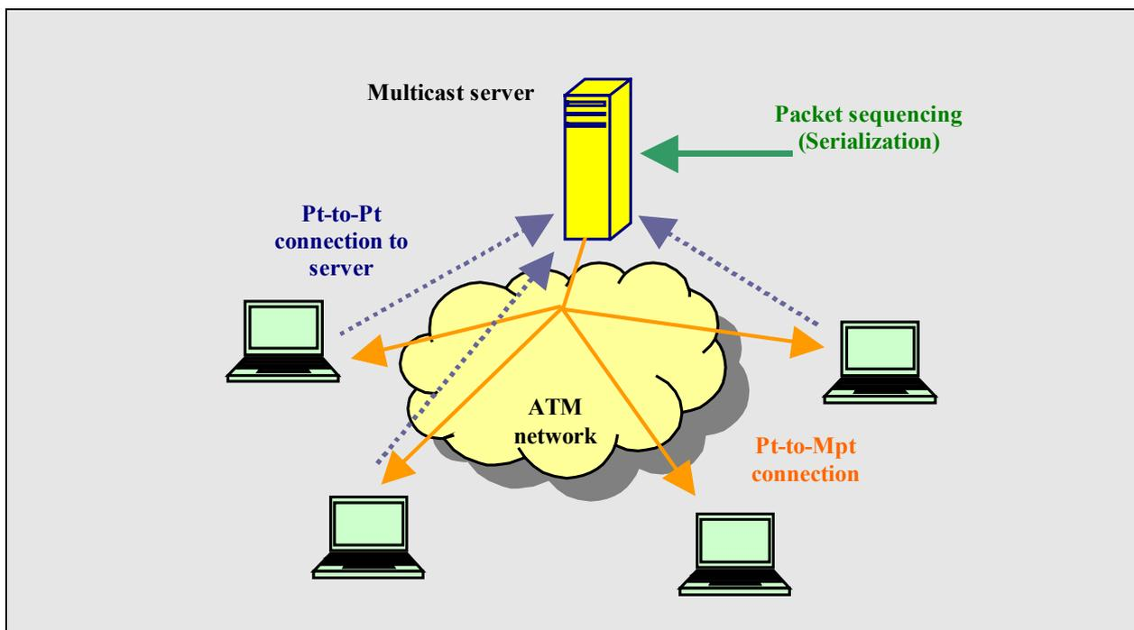
In order to accept different traffic sequences obtained from LANs which rely upon existence of a low level multicast/broadcast capability, ATM requires some form of multicast capability. Three methods have been proposed as solutions:
