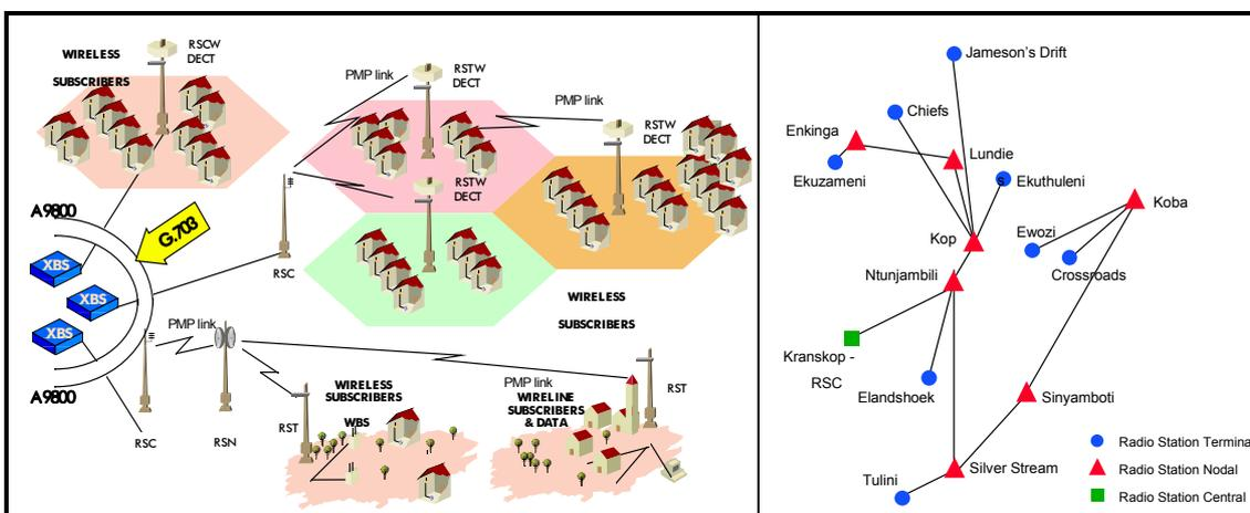
Alcatel is providing 288 000 lines of radio access equipment to the South African operator Telkom. The rural area of Kranskop (see Figure 6) has been selected as a pilot planning application with the objective of the exercise to locate and dimension the Alcatel 9800/DECT equipment. An exchange (Radio Station Central or RSC) serves the whole area via a point-to-multipoint microwave network.
