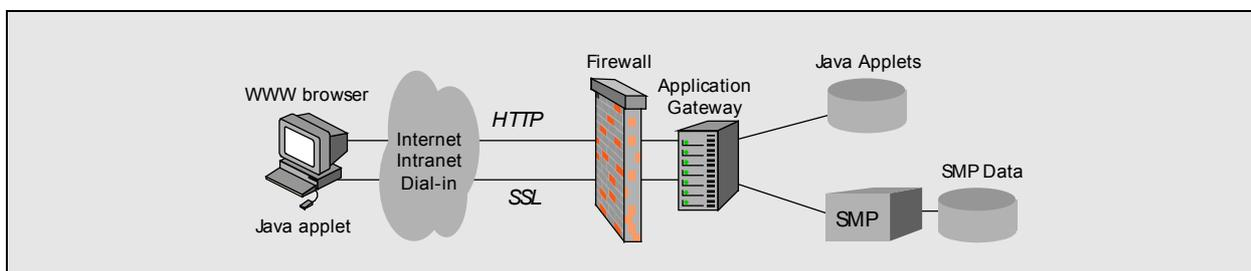
In Figure 2.9.6 the Web interface guides, in a user-friendly manner, the subscriber via hyperlinks and Java applets through the Service logic and data management and Service supervision management.
