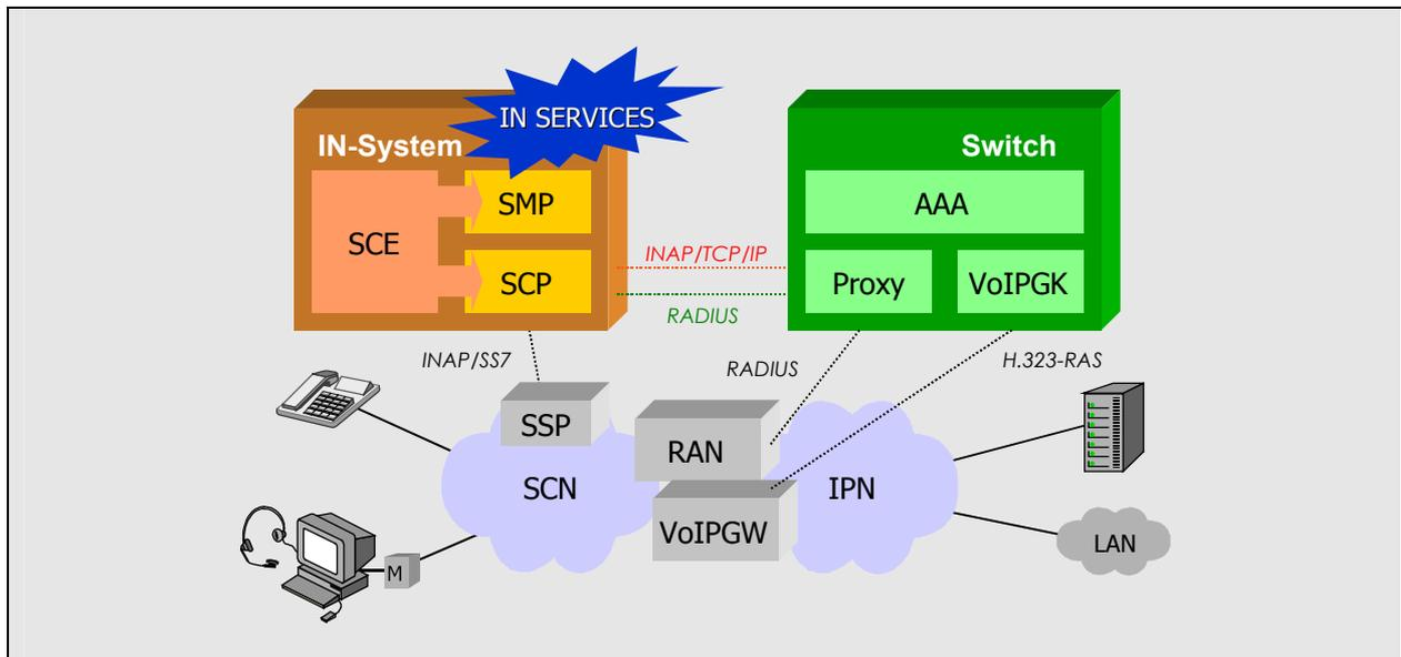
As an short term solution, the proposed interfaces and resulting interworking services are attractive to operators who are also providing Internet access and/or IP telephony services, because it makes optimal reuse of the existing IN platform and services through standardized interfaces between the ISP servers and the SCP.
