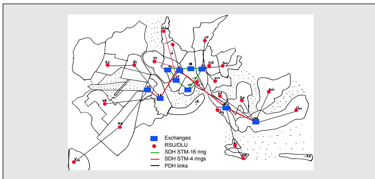
Switching network design led to the definition of a two-level network configuration with ten switches (three new) and an access network consisting of RSUs, DLUs (see Figure A7) and a radio access overlay network.
