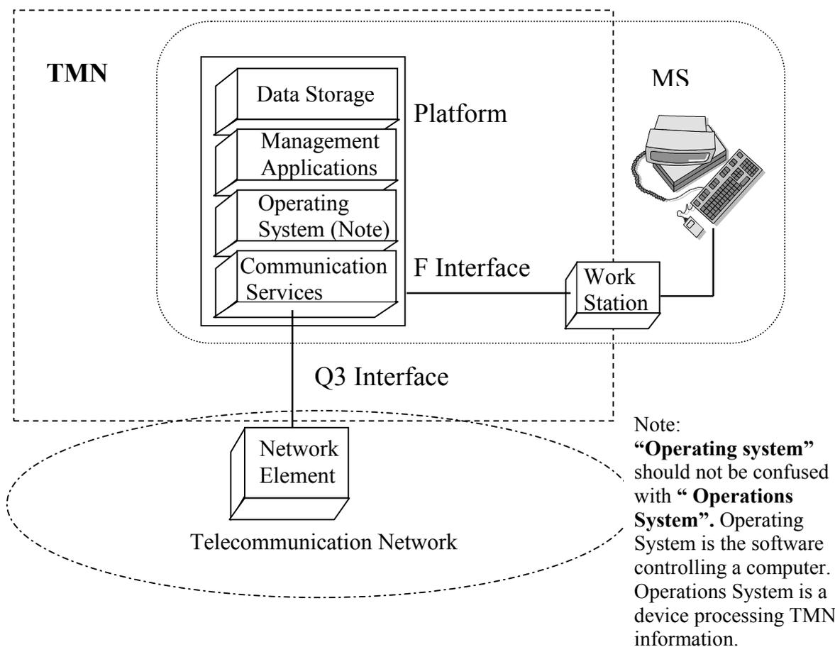
The Management Systems consists of a computer platform and computer terminals, containing:
