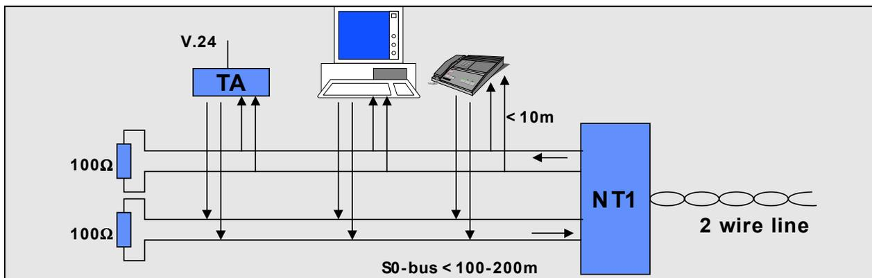
Up to eight ISDN Terminals (TE1) or ISDN Terminal Adapters (TA) can be connected to the  $S_0$ -Bus. Two of them can be used in parallel each accessing one of the B-channels. The terminals may be ISDN telephones, Group 4 Telefaxes or Data-Equipment like a PC with ISDN Adapter-Card. Additionally, terminals may also use the data packet service offered via the D-channel.
