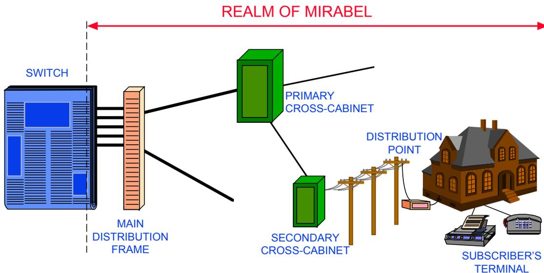
MIRABEL considers copper lines only, since the process is based on electrical tests. Any type of copper wires may be monitored. Even in the case of ISDN lines the wires are tested from an electrical point of view.
