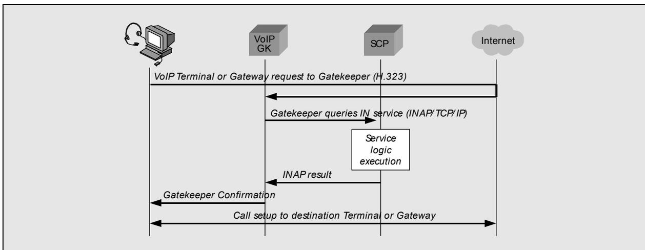
This means, that the function of the Gatekeeper, including the Call Control, will be integrated with the IN platform, as such enriching the basic Gatekeeper functionality (as required by e.g. the H.323 standard) with full-IN features and services, including Virtual Private Networking, Calling Card Services, Interactive Voice Response, Unified messaging, etc.
