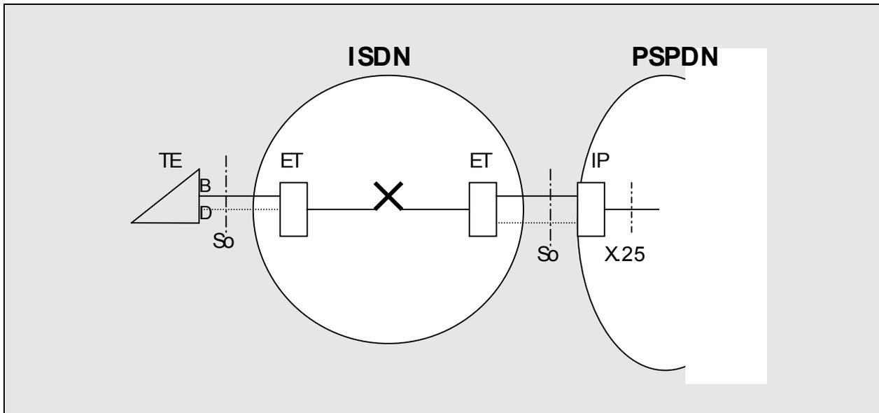
An ISDN terminal, TE, capable of X.25 Protocol or an X.25 DTE adapted to ISDN So-interface, is accessing the PSPDN via B-channel(s) terminating in an ISDN interworking Port unit, IP.
