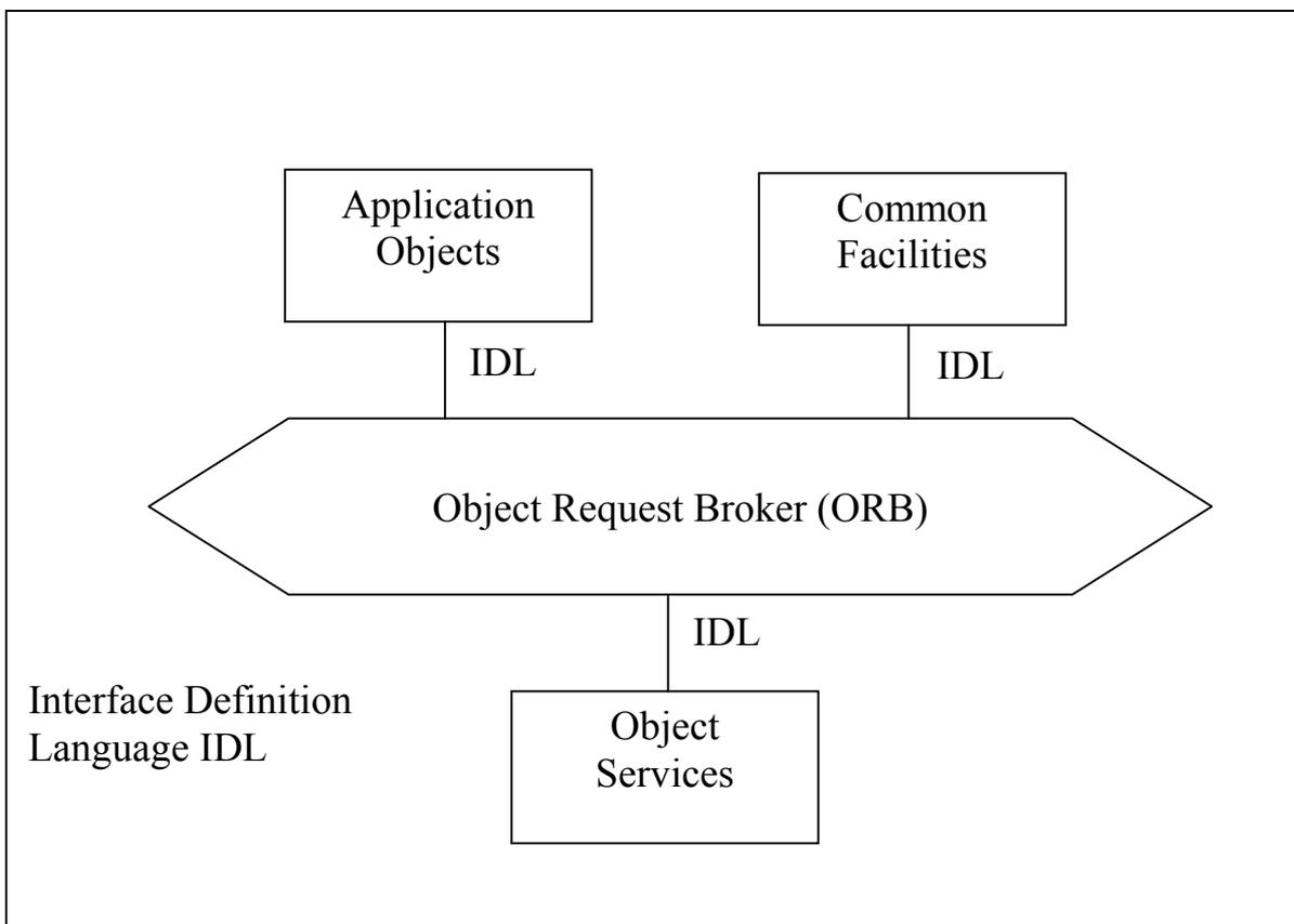
Common Facilities handle User Interface (for e.g. editing services), Information Management (for e.g. document storage), System Management (for e.g. component installation) and Task Management (e.g. workflow and rules). Common Facilities are usable in a general way for different areas belonging to for example telecomms, health service, retail and finance services.
