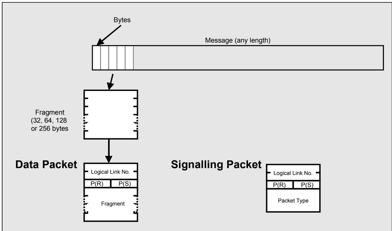
The frames are numbered modulo 8 (standard) or 128 (extended). Frames sent by one extremity of the link must be acknowledged by the other extremity. The procedure offers the possibility of anticipating the acknowledgements: each extremity can send a series of information frames (maximum 7 or 127 according to the case) without waiting for the acknowledgement of the first one. This device avoids dead time between frames and thus transmits at maximum speed.
