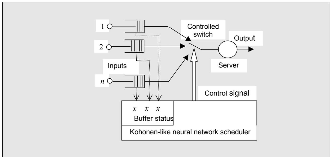
Traffic policing mechanism, based on the NNs, is proven to be more effective than algorithmic ones due to the non-linear and time-varying nature of the traffic. The policing algorithm should be capable of the following: 1) detecting any non-regular traffic situation, 2) selecting the range of checked parameters (i.e., the algorithm could determine whether the user's behaviour is within an acceptable region), and 3) rapid reaction time to any violations in the traffic parameters.
