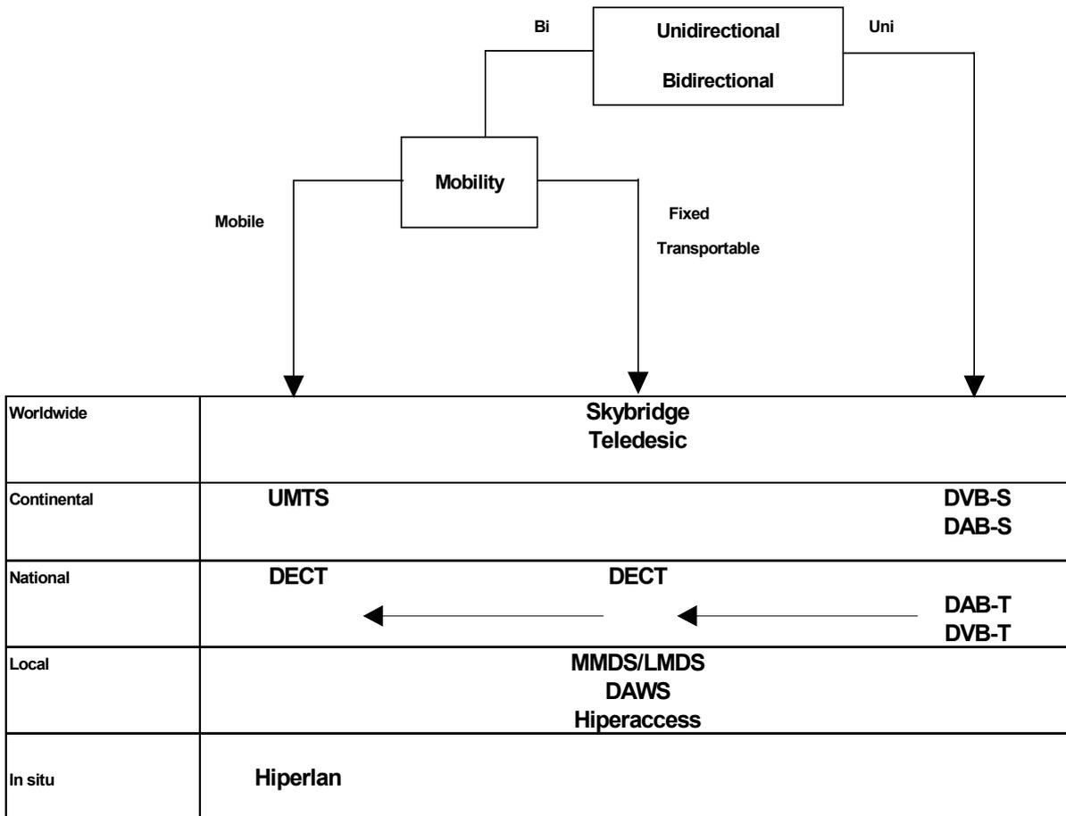
The first applications of wireless access have been to provide basic voice telephony. This application has proven quite successful in lowering the cost of providing telephone service and thus allowing the rapid expansion of teledensity in the less developed nations of the world. With the replacement of voice by data as the driving engine of modern telecommunications, wireless access is rapidly evolving to support ever-higher data rates using packet technology.
