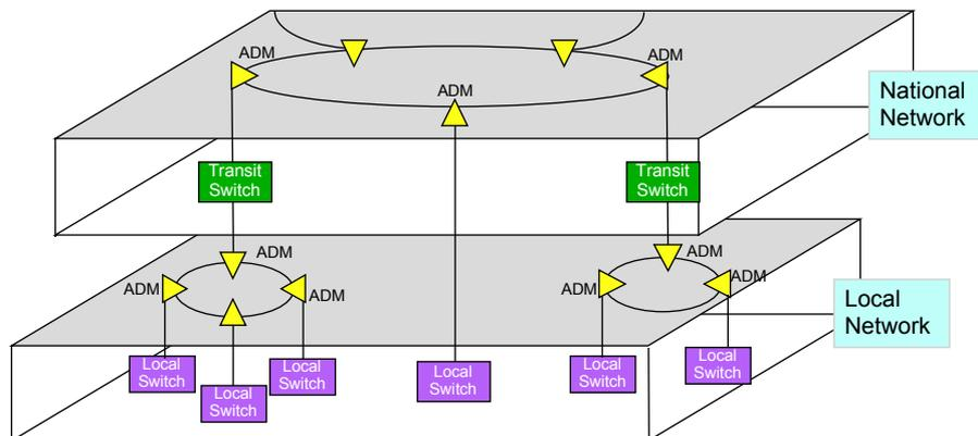
ALCALA supports two network design tasks, the first of which is configuration and topological design. Taking into account the switching configuration and existing outside plant constraints, it selects suitable mesh or multi-ring network structures.
