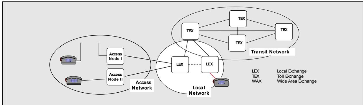
In general, the PSTN is structured as depicted in Figure 2.1.1. The access network has to provide the physical communication link between the communication endpoint and the local exchange. In the local exchange (LEX) all users related functions are located. The switches of the toll exchange level (TEX) are introduced to have the possibility for structuring and optimizing the network according to traffic measurements and user behaviour.
