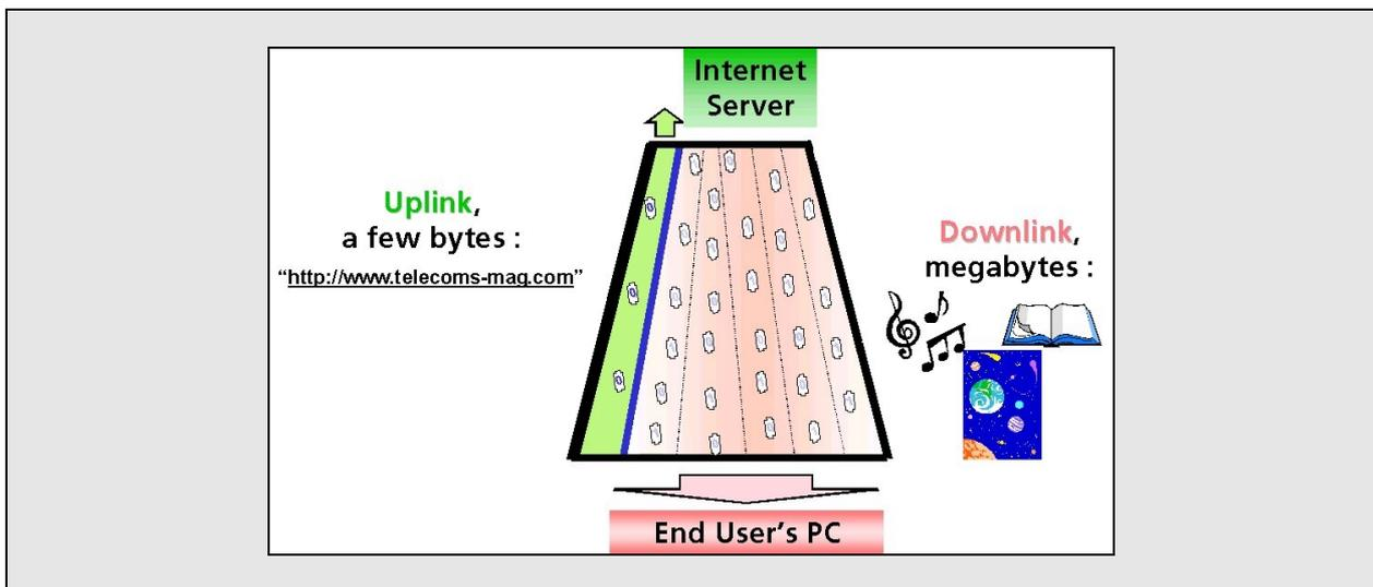
Thus the flow of information in user access to the Internet is commonly quite *asymmetric* in nature. Radio technologies that can dynamically adapt to asymmetry have a distinct advantage over those that do not. In particular, if the duplexing of two-way communications is achieved by means of time division duplex (TDD), it is significantly easier to adjust to asymmetry *in real time* than with frequency division duplex (FDD).
