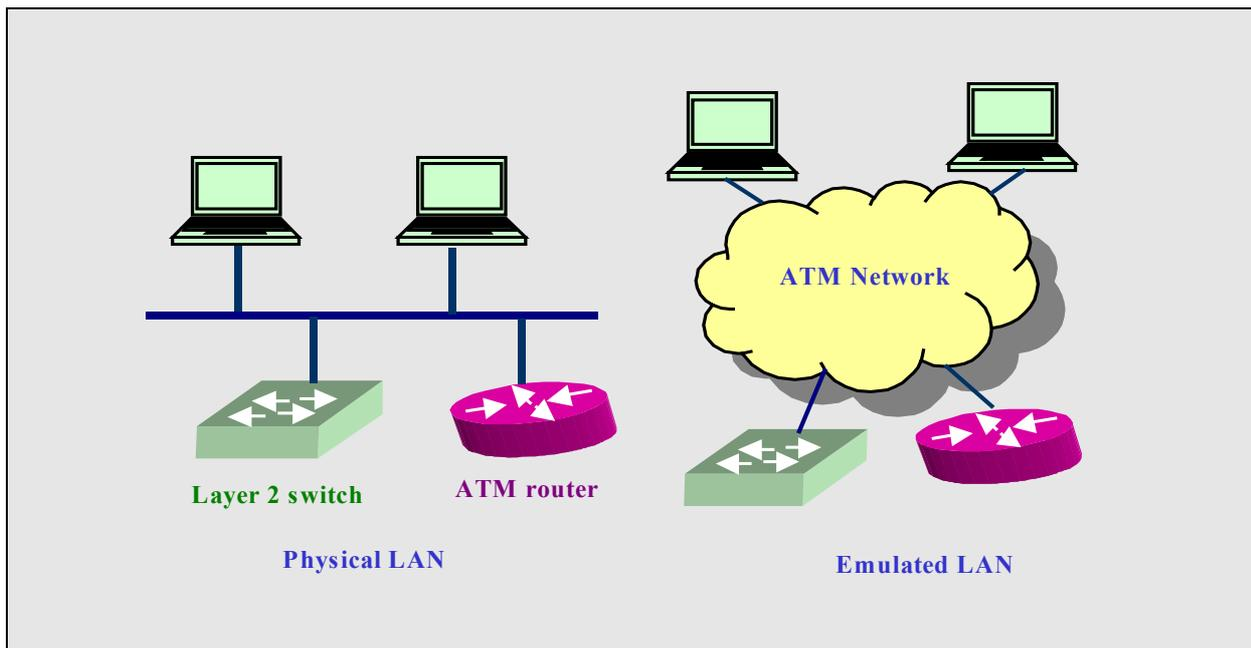
In other words, the LANE protocols make an ATM network look and behave like an Ethernet or Token Ring LAN – although one operating much faster than a real such network.
