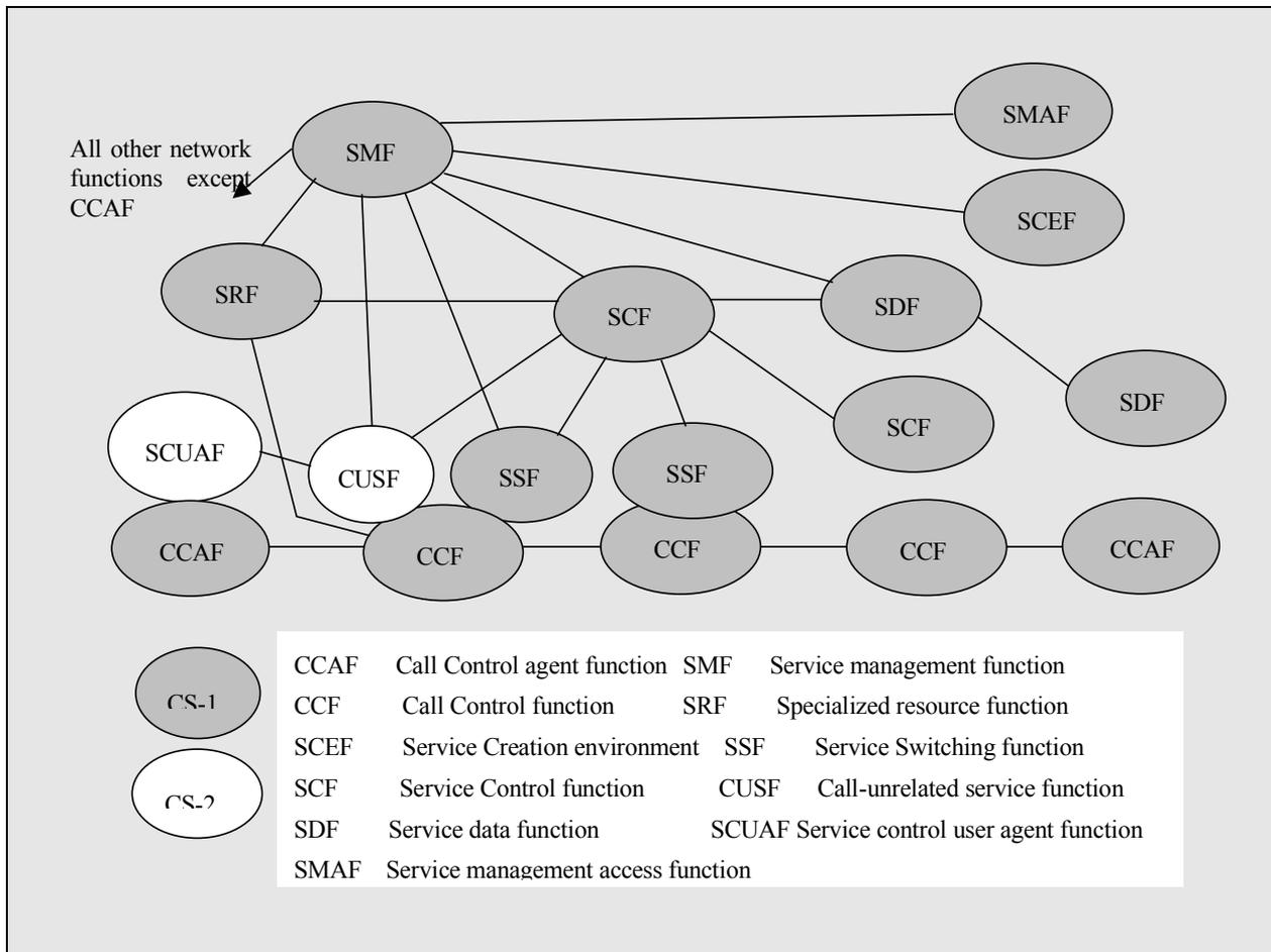
Intelligent Network Capability Set 1 (IN CS-1) (see Table 2.3.1) is the first standardized stage of the intelligent network (IN) as an architectural concept for the creation and provision of telecommunications services.
