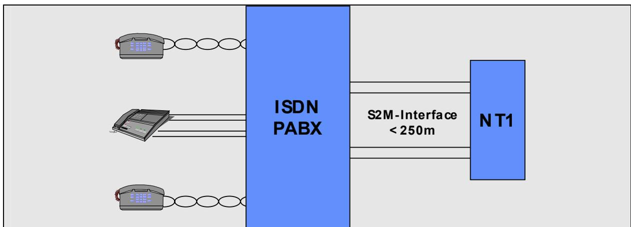
Due to the point-to-point characteristics of the interface no D-channel access mechanism is necessary. It is possible to con the 30 B-channels into bundles using only part of the 30 channels or to assign channels as incoming or outgoing channels only. 2.2.6 shows the channel structure at the S<sub>2M</sub>-interface
