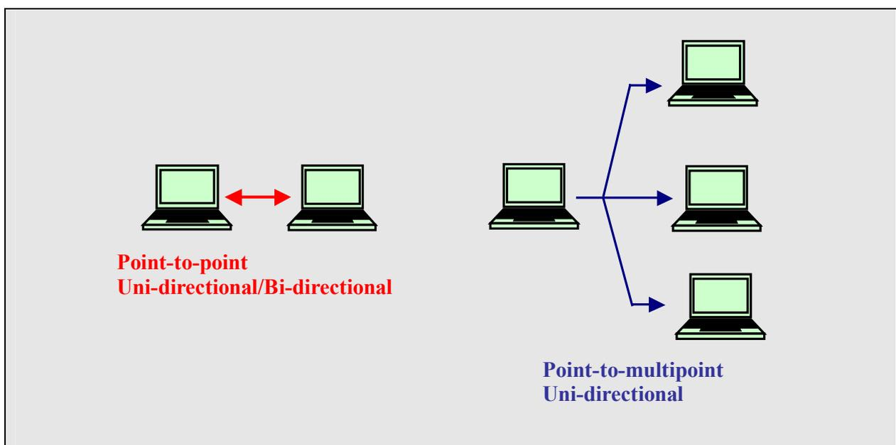
Point-to-multipoint connections are unidirectional, meaning that the root is allowed to transmit data to the leaves, and not leaves to the root or to each other.
