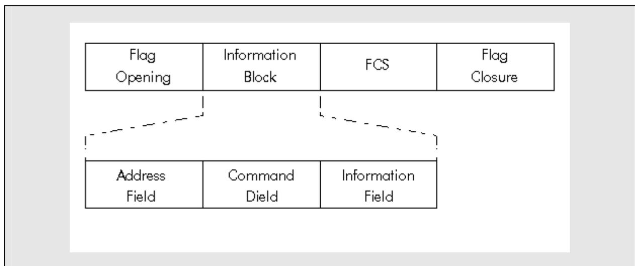
All the frames must start and end with a frame delimiter sequence called the flag (Figure 2.4.5). The flag is used for frame synchronization. The flag is the only frame element that can contain six consecutive 1s. If the user data should generate such a sequence, the procedure automatically inserts a 0 after the fifth 1.
