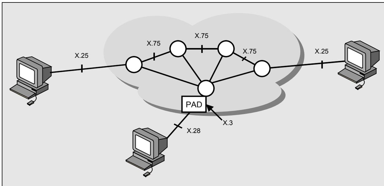
A DTE can be a terminal that does not implement the complete X.25 functionality. A DTE is connected to a DCE through a translation device called a packet assembler/disassembler (PAD). The operation of the terminal-to-PAD interface, the services offered by the PAD, and the interaction between the PAD and the host are defined by ITU-T Recommendations X.28, X.3, and X.29, respectively.
