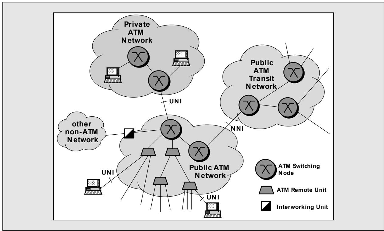
**Broadband ISDN inter-carrier interface (B-ICI)** – defines inter-switch communications in public networks (af-bici-0068.000).
