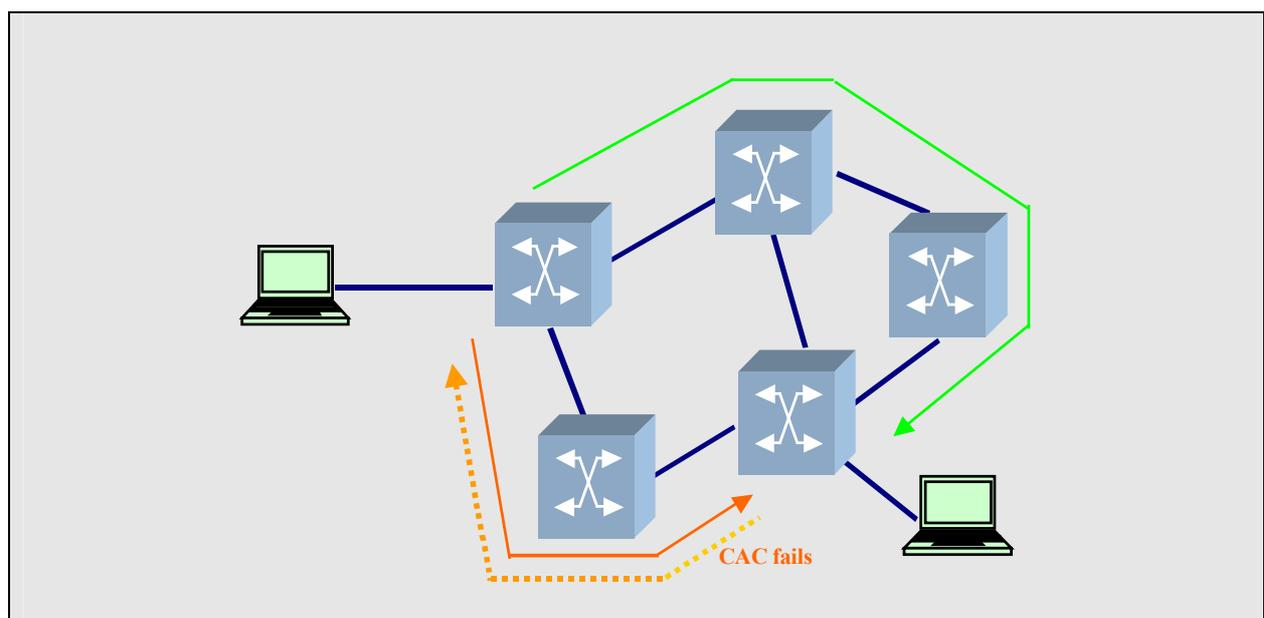
The protocol uses a topology state routing protocol in which nodes flood QoS and reachability information so that all nodes obtain knowledge about reachability within the network and the available traffic resources within the network.
