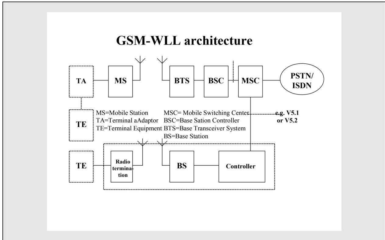
As with analogue cellular, derived fixed digital cellular systems connecting for example the MSC to the PSTN (A1 interface) or a special BSS including a specific controller and connected to the Local exchange via a V5.X interface can be developed. However, even though the price of such equipment may be attractive, the inherent characteristics of the cellular remain.
