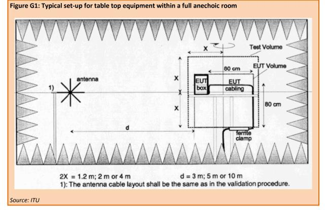
Site validation above 1 GHz normally uses site site-VSWR method, described in the CISPR 16-1-4, of comparing maximum deviations for several antenna positions using both antenna polarizations. To be acceptable the Site VSWR must be less than or equal to 6 dB.
