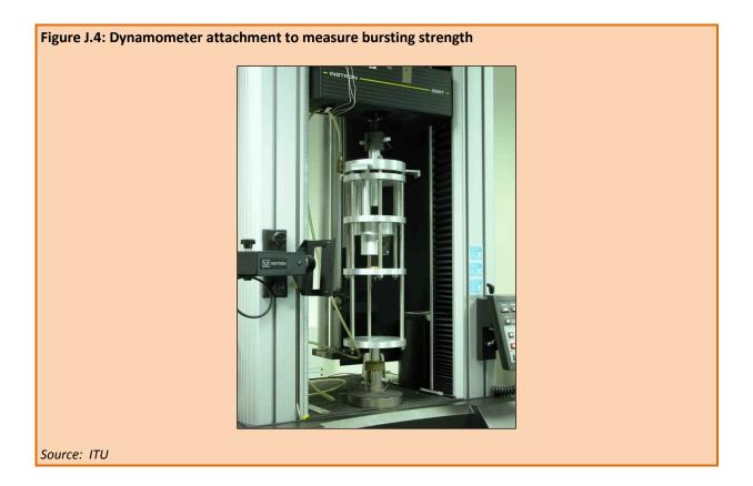
Figure J.4 shows a dynamometer attachment to measure bursting strength of heat shrinkable sleeves used for cable joints. The determination of the bursting strength of rubber- or plastics-coated fabrics according to ISO 3303-1:2012, uses a mechanically operated steel ball.
