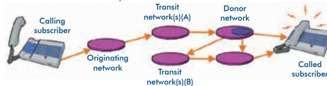
In the above figure, the donor network receives an incoming call. It then detects that the called number has been ported-out to another network and makes a database (DB) query to retrieve a routing number. It thereafter reroutes the call onward towards the recipient network using retrieved routing information. For more information, see: ITU-T E.164 Supplement 2 (11/98).
