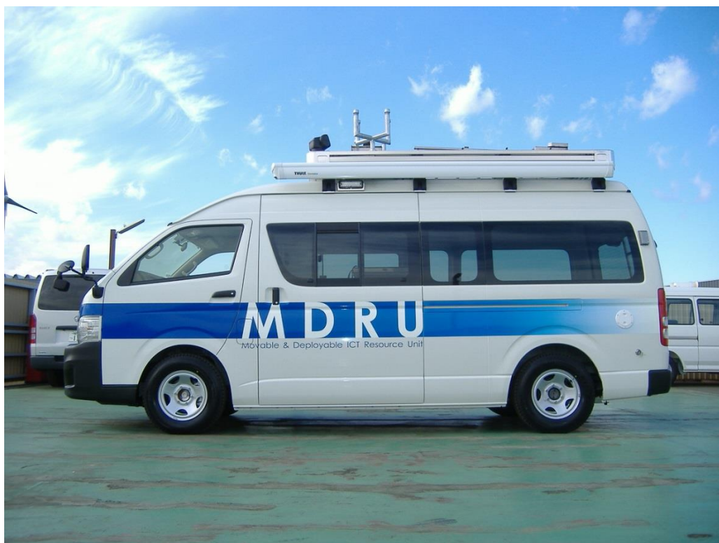
Figure 7 – A van-type vehicle equipped with an MDRU
