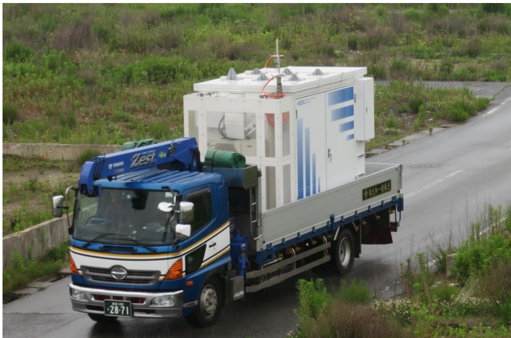
Figure 2 – Transporting an MDRU to a remote site
