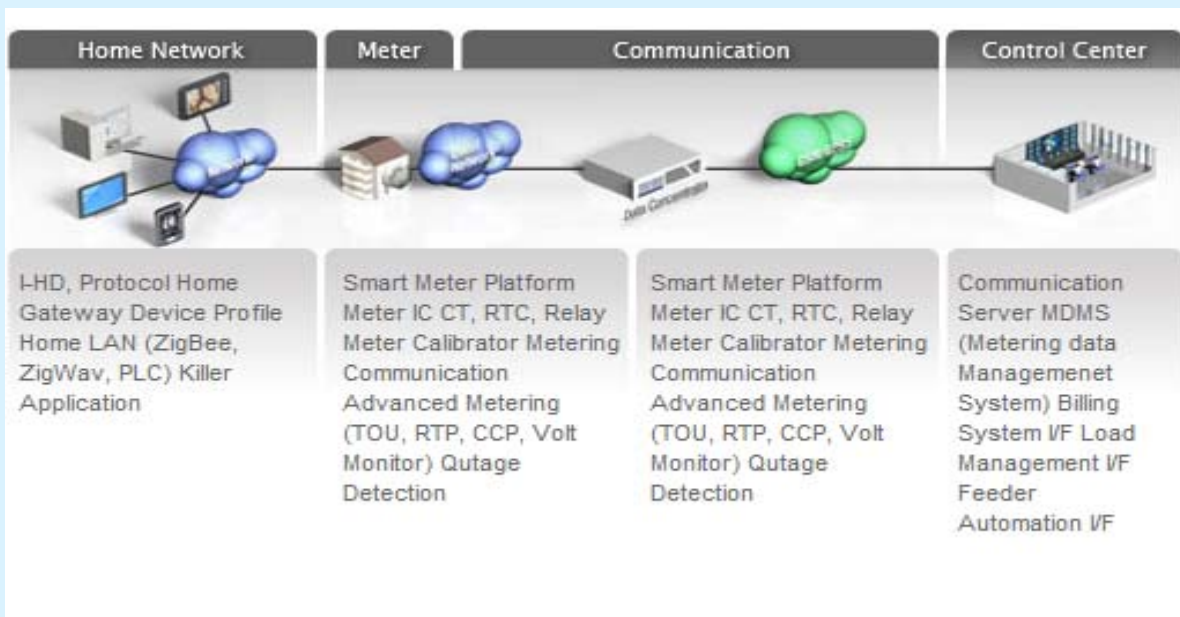
Figure 5 – Components of intelligent remote data collection for smart metering
