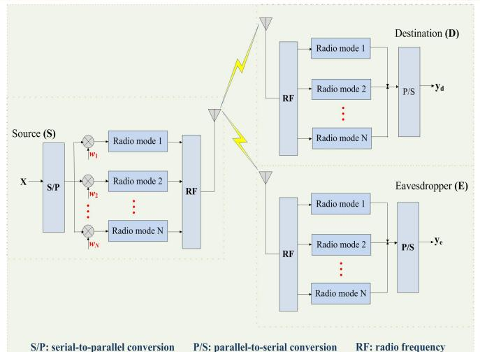
A block diagram of proposed MRC scheme for heterogeneous wireless networks consisting of a source and a destination in the face of an eavesdropper.
