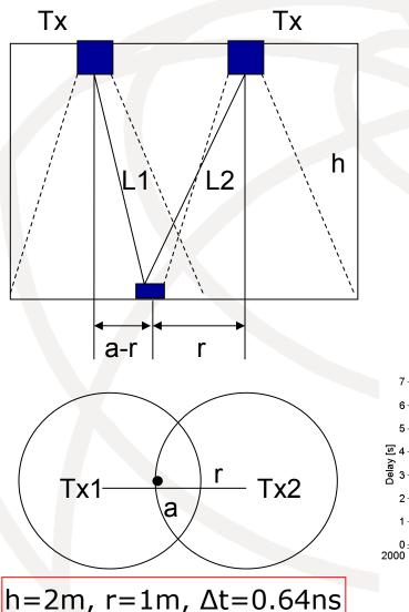
Synchronization in the fiber part can be achieved by path equalizing
