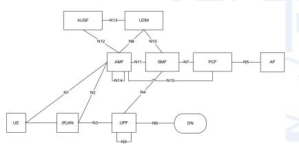
Authentication Server Function (AUSF) Core Access and Mobility Management Function (AMF) Data network (DN), e.g. operator services, Internet access or 3rd party services Network Exposure Function (NEF) NF Repository Function (NRF) Policy Control function (PCF)
