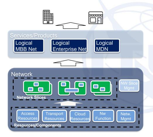
Network slice is a **logical network** serving a defined **business purpose** or **customer**, consisting of **all** required network resources **configured** together. It is created, changed and removed by management functions.
