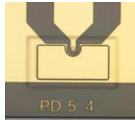
Fabricated untraveling-carrier photodiode
