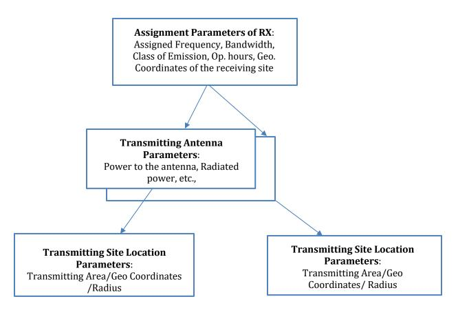
As shown in the above diagram, this notice has the receiving site parameters and two sets of transmitting antenna parameters, with its location. In fact, there is *no* limit concerning the number of transmitting "antennas" for a notice.
