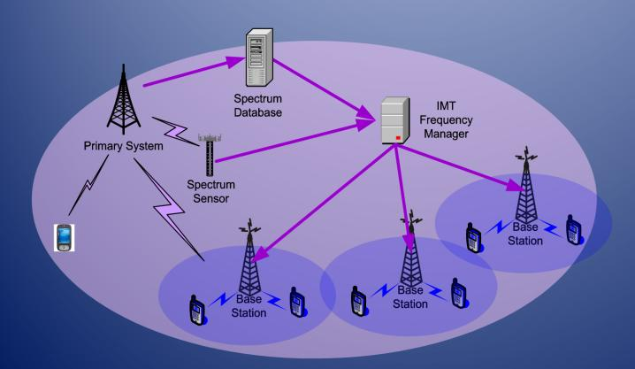
Scenario of IMT with CR functions to sharing the spectrum of other radio system
