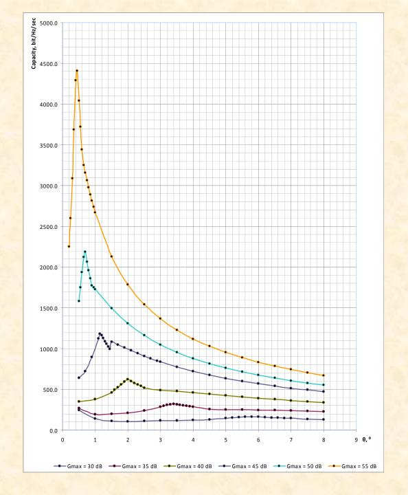
GSO capacity (without taking into account satellite antennas selectivity, only for down-link) amounts from 164 to 4400 bit/GHz/s.
