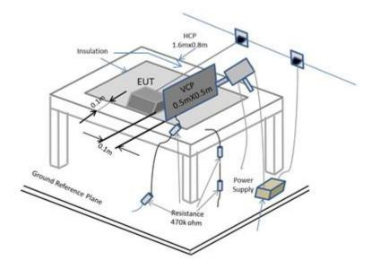
The test setup consists of the discharge generator, EUT and auxiliary instrument necessary to perform DIRECT and INDIRECT application of discharges to the EUT, in the following manner:
