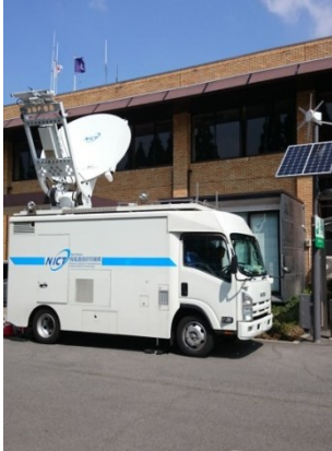
MDRU with NICT's vehicle-mounted satellite base station
