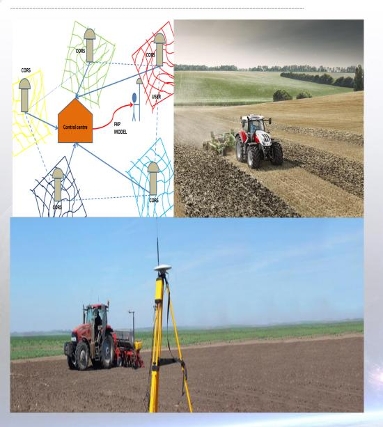
The automatic driving system installed on the agricultural machinery uses Beidou Positioning Technology and remote control technology to divide the farmland into data grid, and farming is strictly carried out according to the set procedure, thus realize the unmanned digitized precision agriculture.
