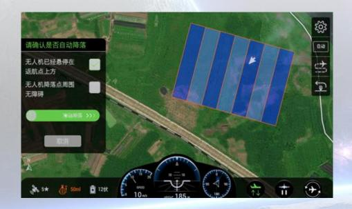
Beidou positioning technology is used to apply agricultural and chemical fertilizers matching the needs of different regions. Once the UAV arrives in the operation area, the system will transfer the basic data of the area to the control platform, so as to achieve accurate positioning and automatic navigation, and then precisely spray drugs according to the designated area.
