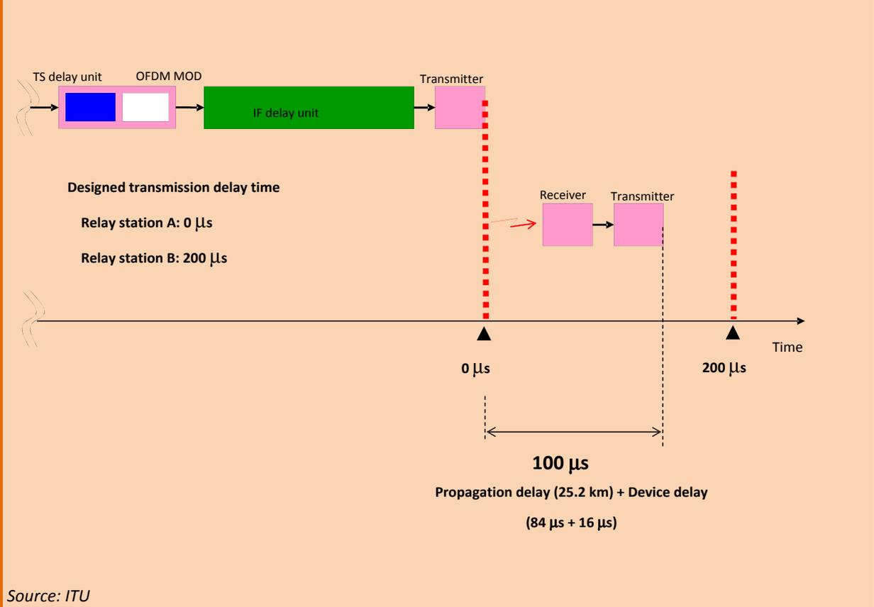
Figure A1.9 (b): Case where transmitting timing is set to 200  $\mu$ s with IF delay unit
