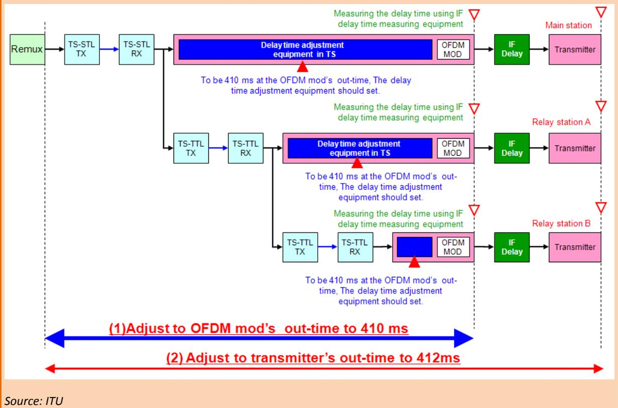
Figure A1.12 (b): Case of delay time adjustment in IF-TTL network
