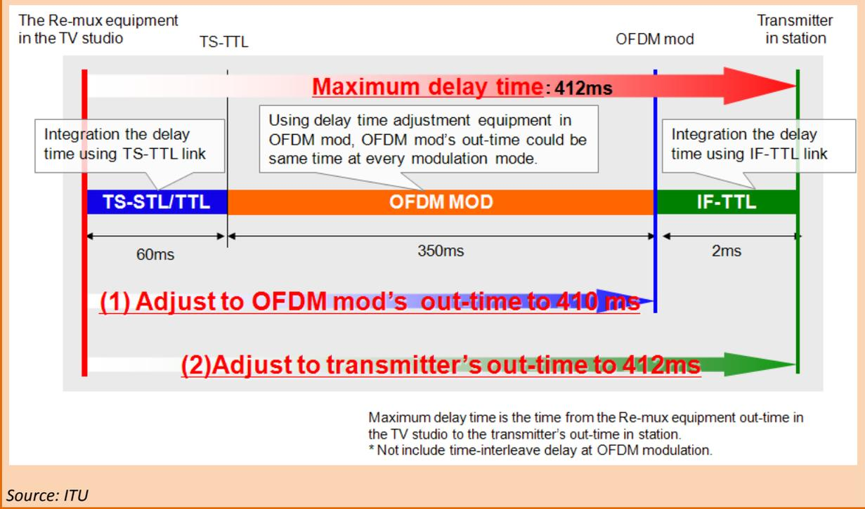
Figure A1.12 (a): Case of the delay time adjustment at TS-TTL network
