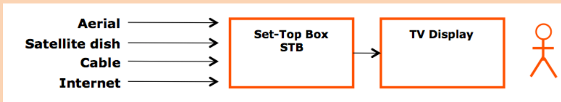
Figure 16: Digital television reception – Set-top box with an existing TV set
