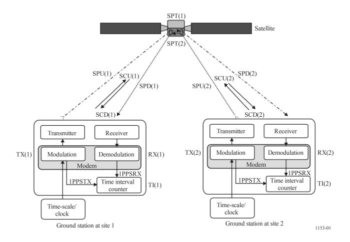
Figure 1 illustrates the various signal delays and explains how the time difference between the clocks at stations 1 and 2 can be determined. The various acronyms have the following significance.
