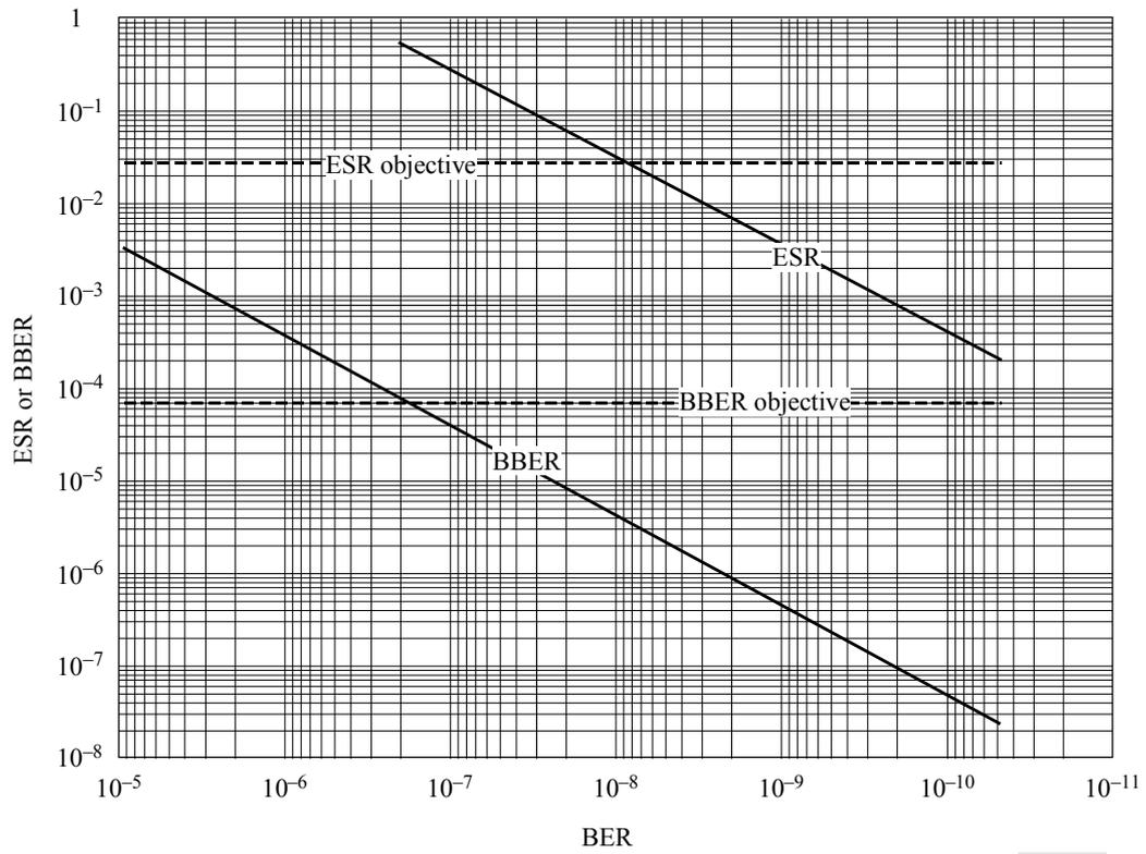
Figure 20 shows ITU-T Recommendation I.356 performance parameters versus BER for IDR (with rate 3/4 convolutional coding and Viterbi decoding). ITU-T Recommendation I.356 objectives are marked.
