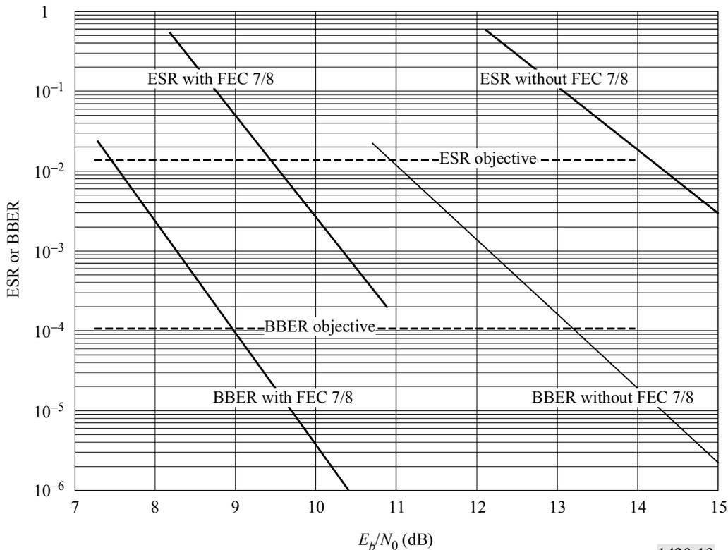
Figure 14 shows ITU-T Recommendation I.356 performance parameters versus  $E_b/N_0$  for the TDMA system. The ITU-T Recommendation I.356 objectives are marked. As in Fig. 13, two sets of results are illustrated. One set is for rate 7/8 BCH coded links, and the other set is for links with no FEC coding.
