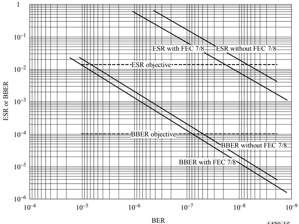
Figure 16 shows ITU-T Recommendation I.356 performance parameters versus BER for the TDMA system. ITU-T Recommendation I.356 objectives are marked.
