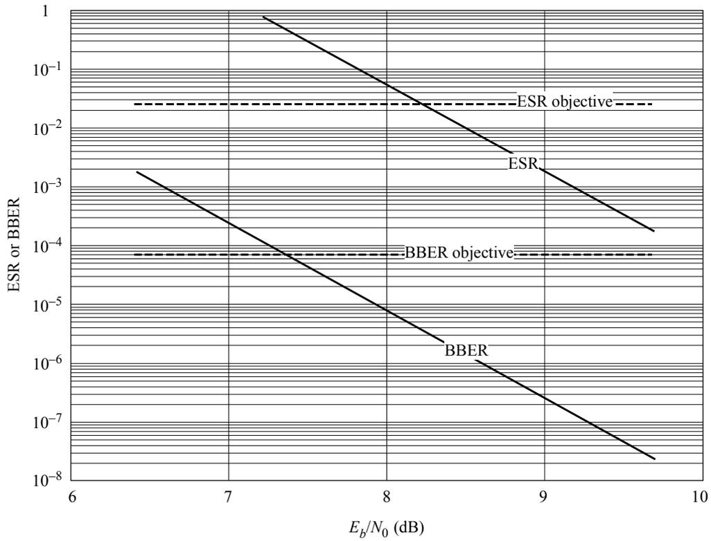
Figure 18 shows ITU-T Recommendation I.356 performance parameters versus  $E_b/N_0$  for IDR (with rate 3/4 convolutional coding and Viterbi decoding). ITU-T Recommendation I.356 objectives are marked.
