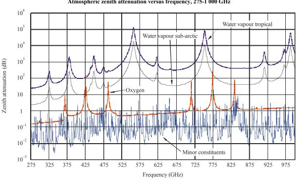
FIGURE 1b Atmospheric zenith attenuation versus frequency, 275-1 000 GHz
