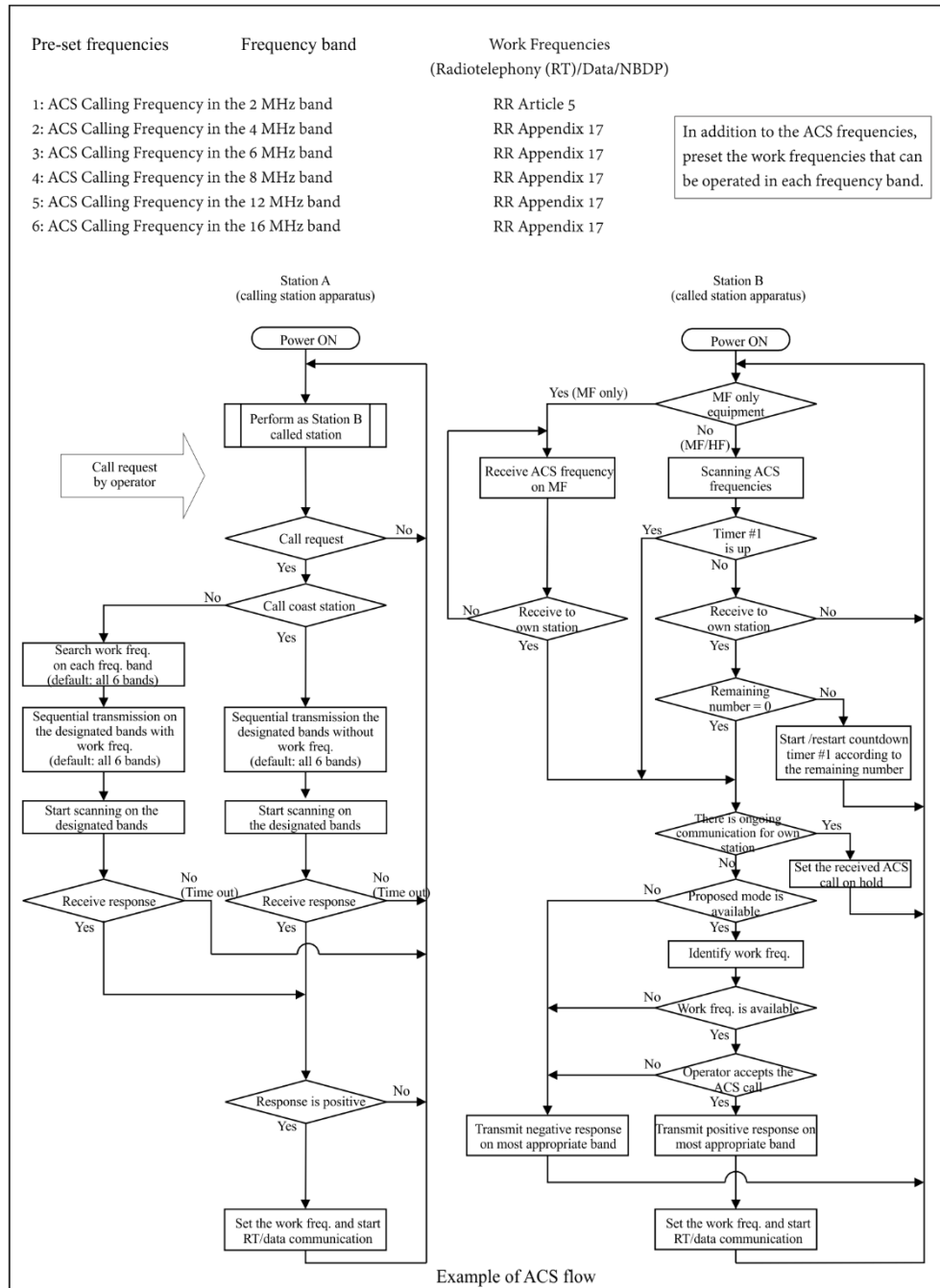
Example of automatic connection system operational procedures
