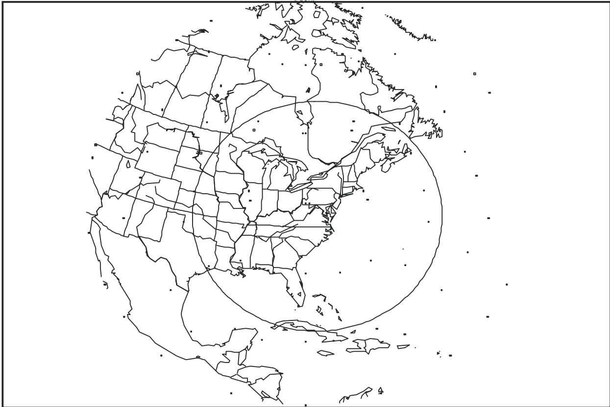
FIGURE 31 Single satellite coverage region, 853 km, 15° elevation angle
