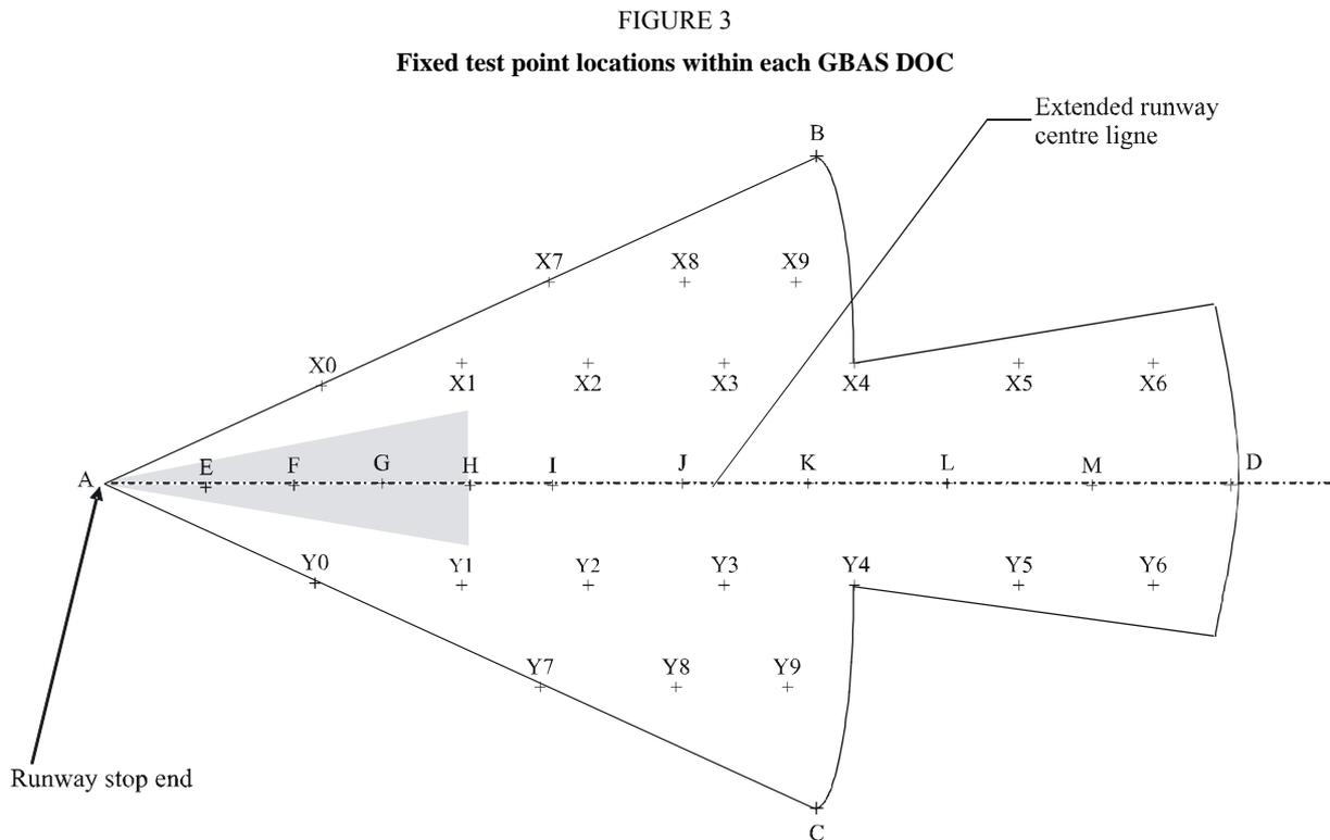
*Note 1* – The shaded zone extends 12 km from the runway stop end and is within  $\pm 7.5^\circ$  of the extended runway centre.
