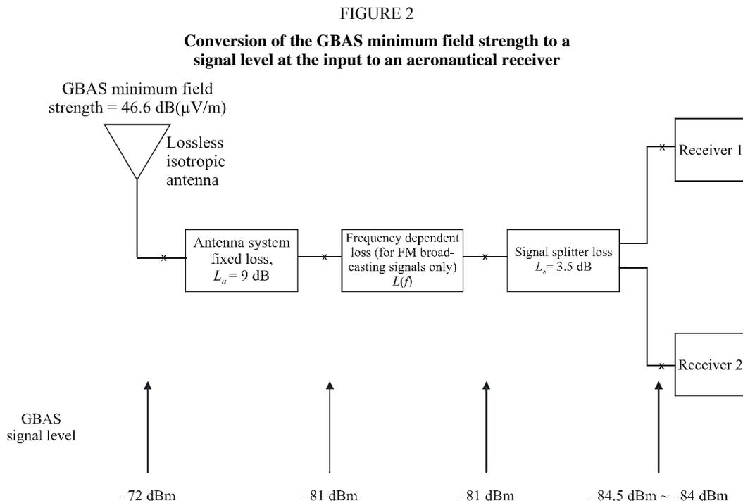
Note 1 – Typical aircraft installation includes a signal splitter to feed two aeronautical receivers.
