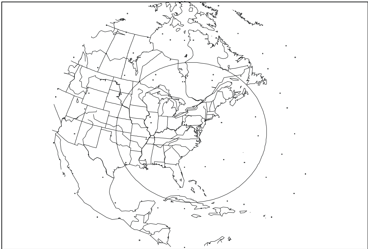
FIGURE 115 Single satellite coverage region, 853 km, 15° elevation angle
