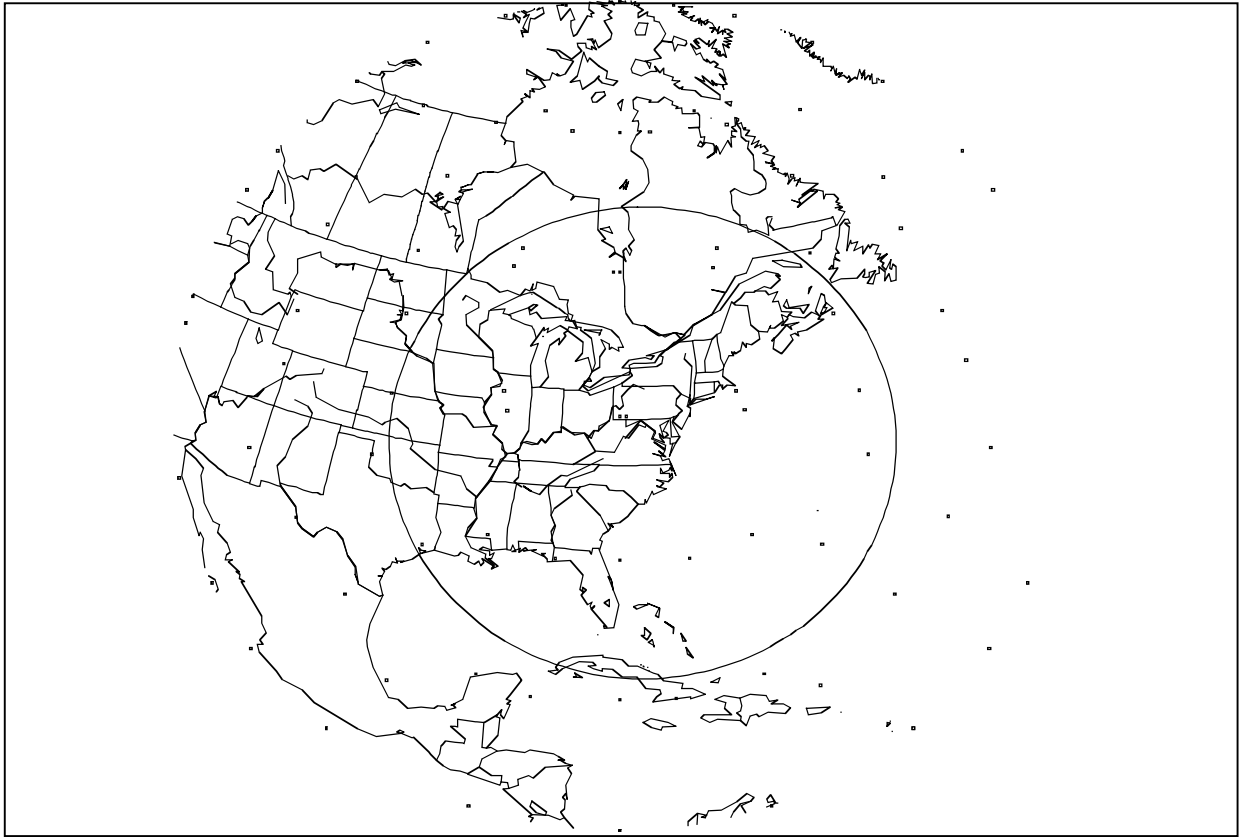
FIGURE 104 Single satellite coverage region, 853 km, 15° elevation angle
