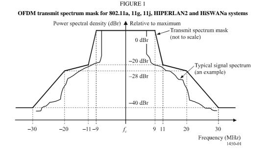
NOTE 1 – The outer heavy line is the spectrum mask for 802.11a, 11g, 11j, HIPERLAN2 and HiSWANa, and the inner thin line is the envelope spectrum of OFDM signals with 52 subcarriers. NOTE 2 – The measurements shall be made using a 100 kHz resolution bandwidth and a 30 kHz video bandwidth.
