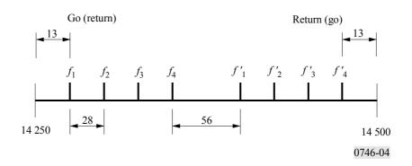
NOTE 1 – Due to the narrow edge and centre guardbands, channels 1 and 4 are unsuitable for use at 34 Mbit/s on a 28 MHz channel spacing. These channels are, therefore, restricted to use for 625-line analogue television or low capacity digital systems, with the channels subdivided to 7 and 3.5 MHz, in a similar manner to that adopted in Recommendation ITU-R F.497, § 10, Alternatives I and III.
