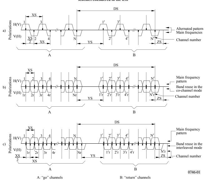
The choice of radio-frequency channel arrangement depends on the values of cross-polar discrimination (XPD) and on the net filter discrimination (NFD) where these parameters are defined as:
