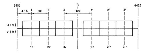
$f_0$  (centre frequency) = 6 137.5 MHz Symbol rate = 74 MBd X = 1.22 Y = 1.62 Z = 0.64
