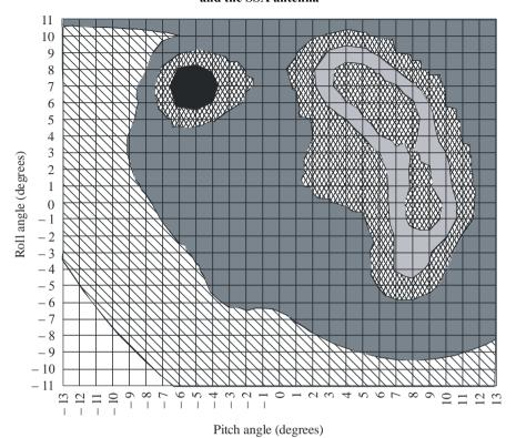
DRS longitude =  $-41.0^{\circ}$ DRS latitude =  $0.0^{\circ}$ FS antenna gain = 33.0 dB Maximum interference to SSA = -150.7 dB(W/kHz)
