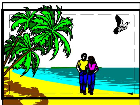
4:3 image as seen in camera and on standard display showing proposed camera viewfinder graticules for 14:9 framing and 14:9 action area (90% of the width/height of the 14:9 framing area).
