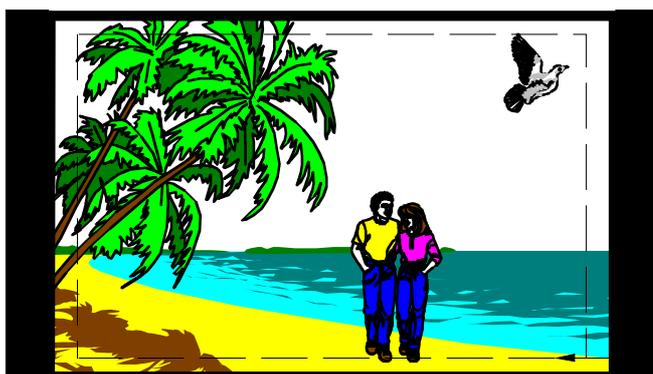
Example 4 - 16:9 image format extracted from 4:3 source showing the residual horizontal 14:9 framing and action area. Small black bars at the sides.
