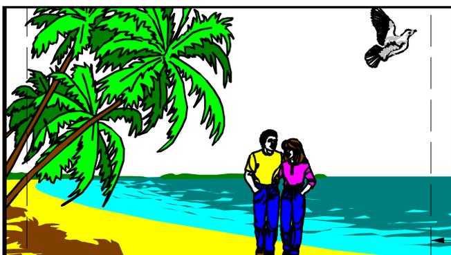
Example 3 - 16:9 image format extracted from 4:3 source showing the residual horizontal 14:9 framing and action area. Original image width retained, height cropped to approx. 14:9 action limit. No black bars.
