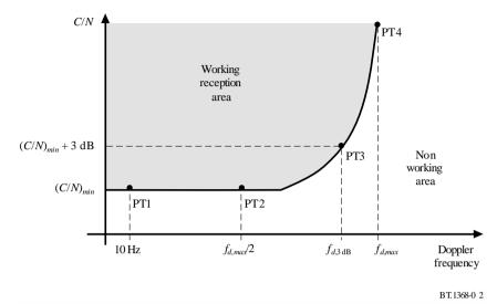
The minimum required average C/N values  $(C/N_{min})$ , Doppler frequency for an average C/N equal to  $C/N_{min} + 3$  dB and the maximum Doppler (speed) limits for mobile reception without diversity are given in Tables 121 to 123. The speed limits for  $C/N_{min} + 3$  dB are given for four frequencies (65 MHz, 200 MHz, 500 MHz and 700 MHz). The average C/N value,  $C/N_{min} + 3$  dB, is suitable for calculation of required field strength.
