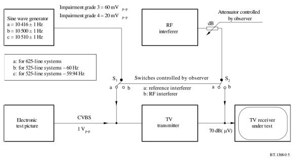
The intensity of the RF interferer can be changed with an attenuator controlled by the observer. The RF interferer is adjusted to produce the same impairment grade as the reference interferer by comparing the interfered pictures on the TV screen.
