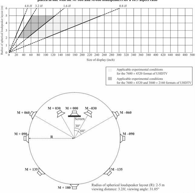
Relationship between the radius of the spherical loudspeaker layout and the size of the video display screen placed in line with the M+060 and M-060 loudspeakers for a 16:9 aspect ratio
