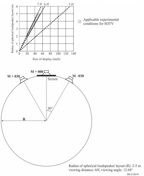
Relationship between the radius of the spherical loudspeaker layout and the size of the video display screen placed in line with the M+000 loudspeaker for a 4:3 aspect ratio (SDTV)
