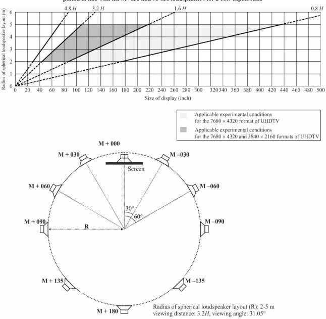
Relationship between the radius of the spherical loudspeaker layout and the size of the video display screen placed in line with the M+030 and M-030 loudspeakers for a 16:9 aspect ratio
