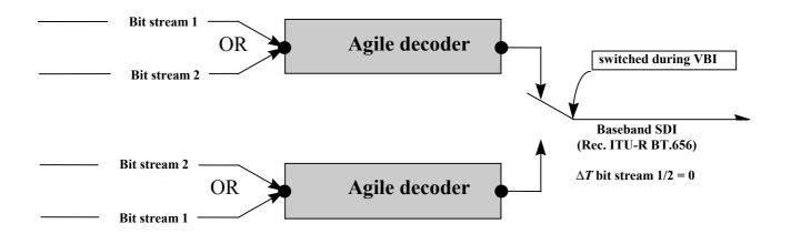
b) Intra-family switching between different bit streams at the input.
