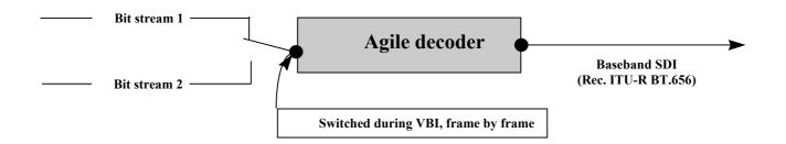
NOTE 1 – As an example, bit stream 1/2 in the above block diagrams could be: DV-based 25 Mbit/s (4:2:0 or 4:1:1) or DV-based 50 Mbit/s within the DV family or MPEG-2 based 422P@ML, 18 Mbit/s, IB or MPEG-2 based 422P@ML, 50 Mbit/s, I within the MPEG family.
