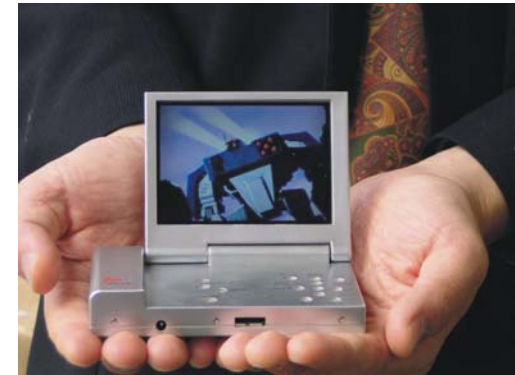
FIGURE 3 An example of enhanced handheld receivers for digital BSS (sound)
