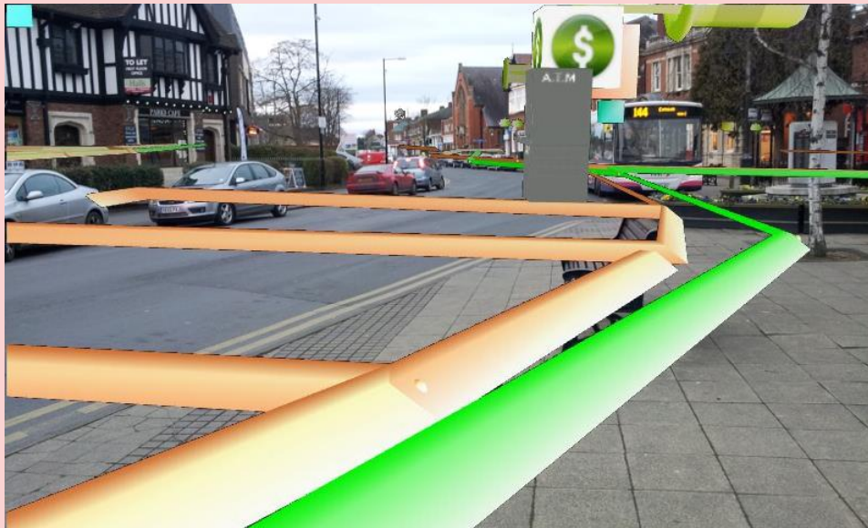
Figure 4: Awila Augmented Reality browser transfers geospatial data from a Web service to the mobile client and overlays the real world with useful digital information (Figure from Augmented Technologies)
