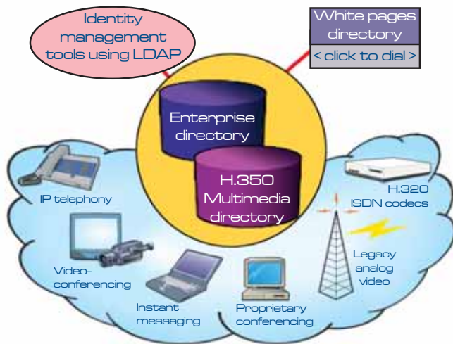
H.350 allows multiple applications, call servers and protocols to access the same master directory information source
