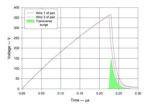
Existing SPD voltage measurements don't cover the generation of transverse voltage surges by the asynchronous SPD operation. Ethernet ports typically have a transverse surge capability below 10 volts and it is important to characterise any SPD intended for Ethernet protection for the level of transverse surge generated.
