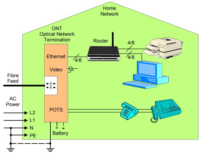
Alternative configuration: (O)NT feeds a Home/Residential Gate-Way outputting Ethernet, POTS and Video
