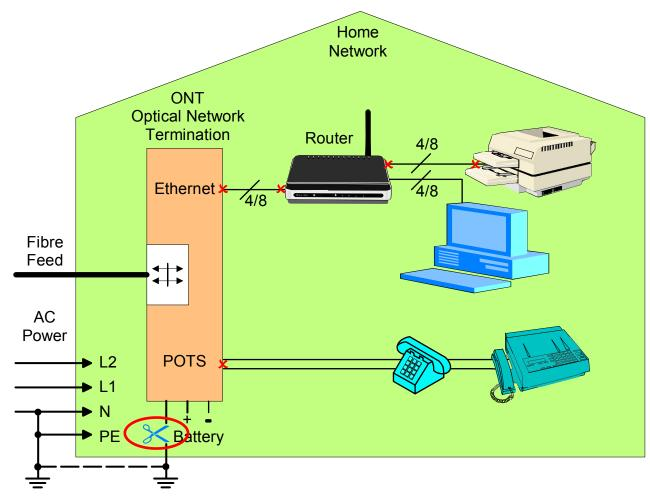
• Disconnecting ONT grounding lead greatly reduces failures, but may cause EMC problems
