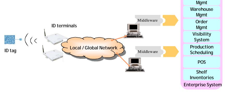
(\*) including NID based on RFID (using radio waves to identify objects)
