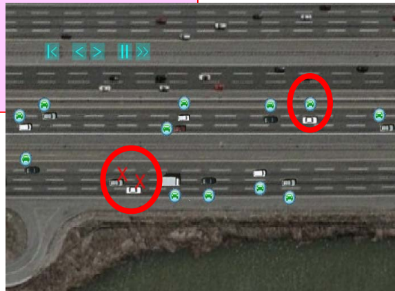
Each vehicle receives a small amount of data from RSU (some vehicles receive nothing due to shadowing, etc)
