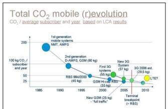
Figure 7: Reduction of CO2 emissions per subscriber in successive generations of mobile phone
