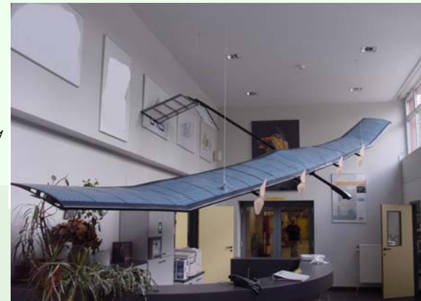
Mercator-1 prototype : ~16 m wingspan, ~2 kg payload (VITO)
